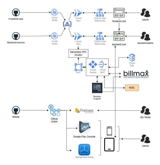
This diagram depicts a cloud based application ecosystem, showcasing the deployment and interaction of frontend and backend web services through Google Cloud's infrastructure, including load balancing and serverless VPC access, alongside a mobile application deployment pipeline utilizing GitHub Actions, Firebase and platform specific distribution channels, all interconnected and integrated with external services like Billmax and Amazon Cognito.
