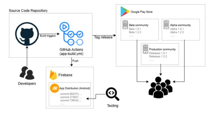
The diagram demonstrates a software release process that uses GitHub Actions to trigger builds when developers commit code to a repository. Firebase App Distribution then distributes these builds to the Alpha, Beta and Production communities within the Google Play Store. This allows for testing at different stages and controlled release of the Android application.
