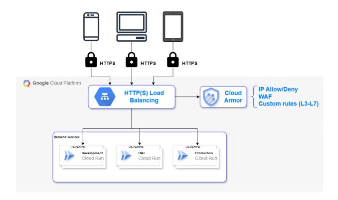
The diagram illustrates a Google Cloud Platform architecture where user devices securely access Cloud Run services (Development, UAT, Production) through an HTTPS Load Balancer, protected by Cloud Armor for IP filtering, WAF and custom rules.
