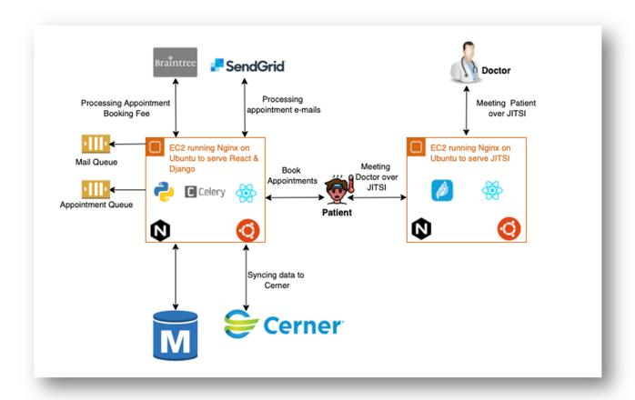
(Architecture diagram shows use of AWS services for the solution.)
